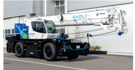
Tadano's electrified rough terrain crane EVolt eGR-250N is already available for the Japanese market
